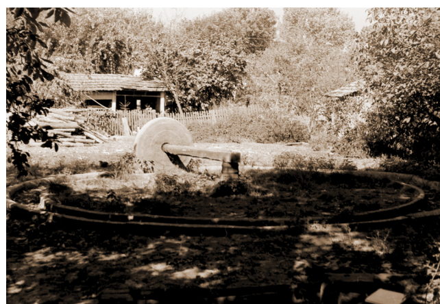
Fig. 7. Apple fermentation in Hungary: apple fruits were smashed with a special machinery similar to a mill wheel called almatörő járgány (apple-cracker capstan). (Picture is from the archive photo gallery of Janus Pannonius Museum, Pécs, Hungary).
